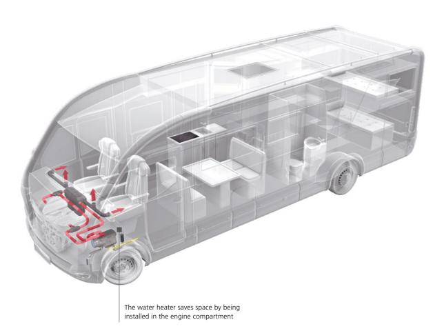
The Thermo Top Evo can also be integrated into the existing water heating system.
