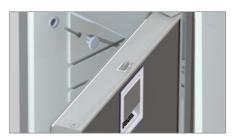
The installation system allows an easy fixing of the cabinet directly from the interior of the fridge. An external flange is not necessary for the installation. An innovative internal bushing structure prevents the crushing of the insulated side wall.
