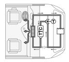
When the cabin is warm enough, the thermostat valve opens and the engine is also heated up by the hot water. The effect can even be increased by reducing the blower speed at the air outlets
